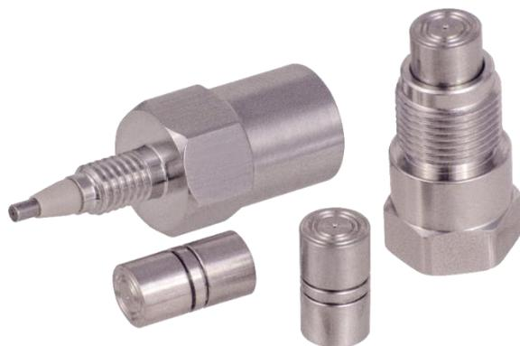
Protection can be perfectly ensured by installing a pre-column filter holder with a 0.2 $\mu$ m or 0.5 $\mu$ m frit. This in-line filter can withstand pressures of up to 1375 bars and is easy to use. The filter holder consists of a two-piece body and replaceable filter – a metal frit.
